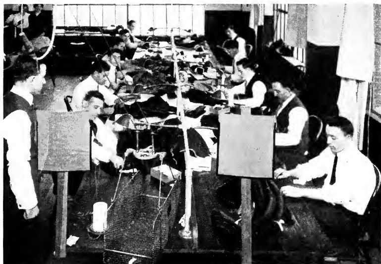
In the factory of the Kahn Tailoring Company baskets run by trolley from the central control station to the work tables, where different parts of a suit are made. Each day's allotment of work has a separate set of compartments in the semi-circular rack above. Colored signals at each table indicate what day's work is in progress. The aim is to get tomorrow's flag up before the whistle blows today
